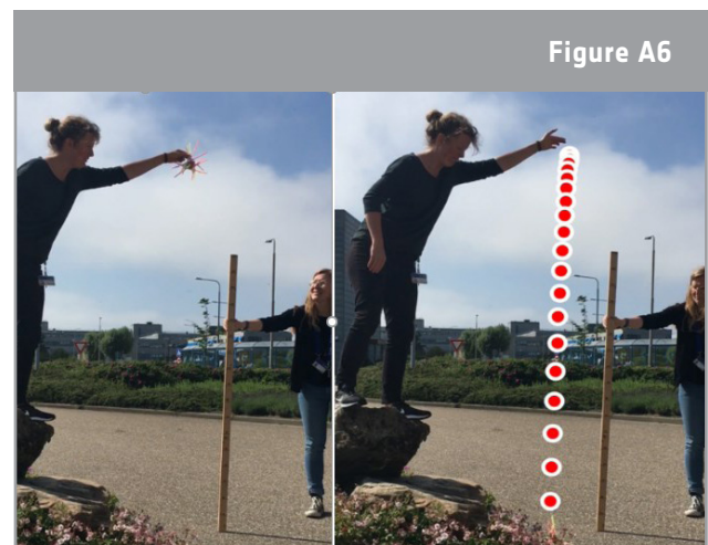
↑ Example of a test drop video motion analysis from approximately 2 m height.
