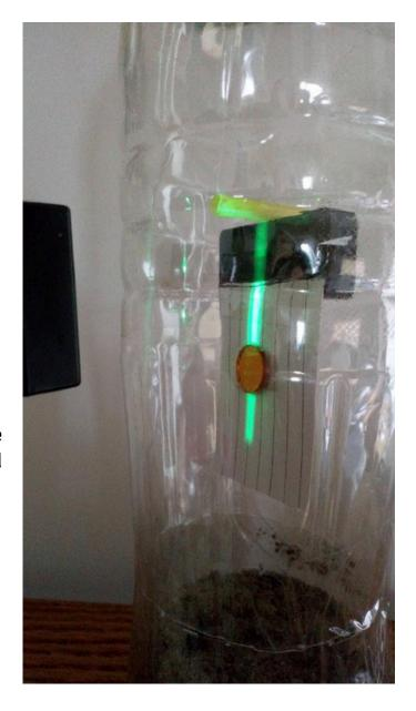
If the Earth's magnetic field changes due to a solar storm, the magnet will move very slightly. This will move the mirror and the dot of light on the wall will change position.
